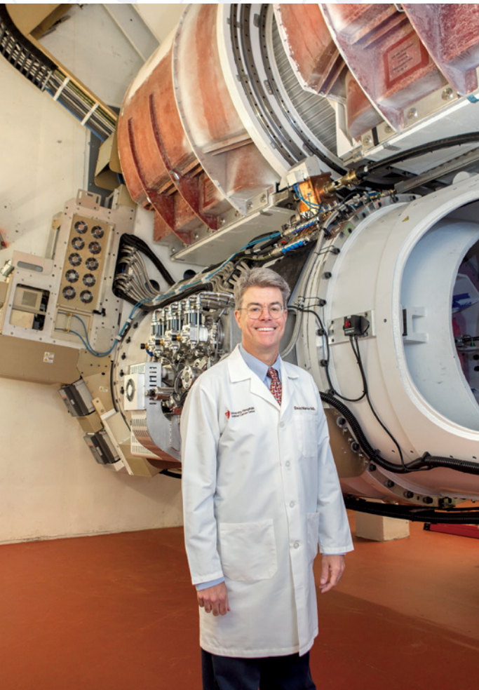
University Hospitals is one of the first in the world to install the Mevion S250. This unique single-room system requires only a 40-foot long by 40-foot wide by 40-foot tall space — significantly less than traditional proton therapy systems which are the size of a football field. Yet it is equal in power. Dr. David Mansur is shown here with the gantry-mounted superconducting synchrotron.
