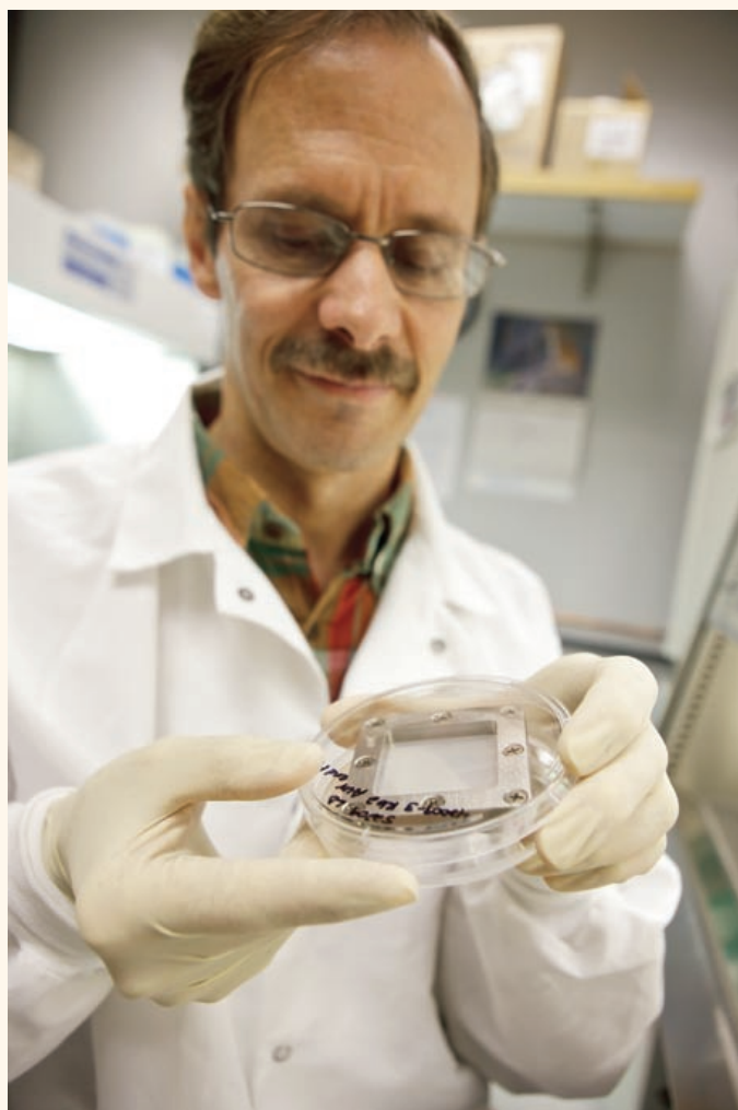
James Dennis, PhD, heads the Tissue Engineering Laboratory in the Department of Orthopaedics at Case Western Reserve University. He holds a bio-reactor (above) invented in his laboratory to grow cartilage (below).
